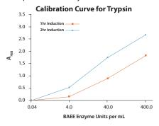
Figure. Calibrator cuvres generated using the PDQ<sup>TM</sup> Colorimetric Assay. Trypsin was at 400, 40, 4.0, and 0.4 BAEE Units/mL incubated for 1 or 2 hours.
